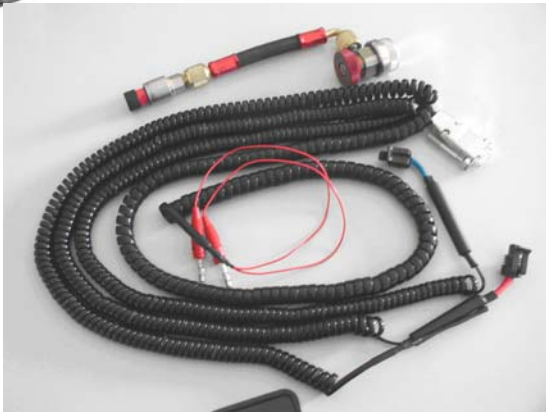
Electronic pressure sensors from diagnostic kit.
