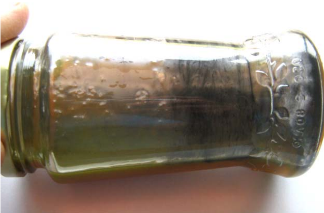
Contaminated PAG oil from a system with a worn compressor.
