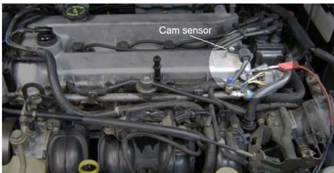
Picture 6: Engine bay with cam sensor highlighted
