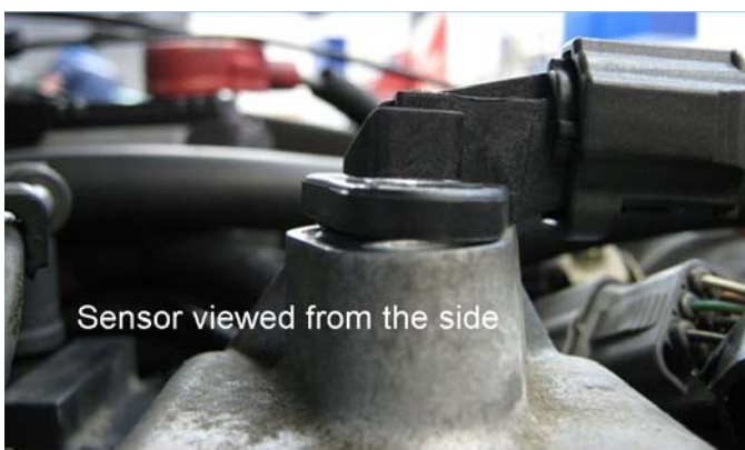
Picture 7: Cam sensor sits in a funny angle, (also with the bolt in) could this be why there is a signal offset?
