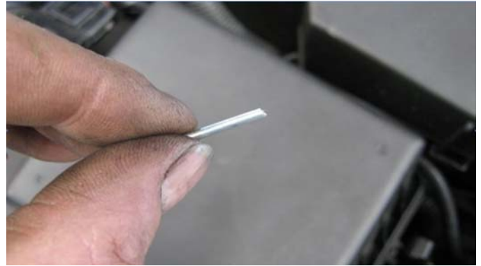
Picture 8: Split pin tab removed from under the base of the cam sensor!
