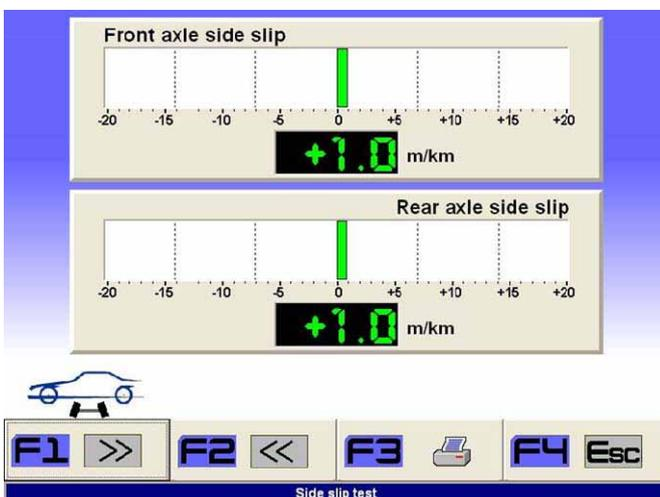
*Reduced camber, with correct toe, but driving in reverse direction.*
