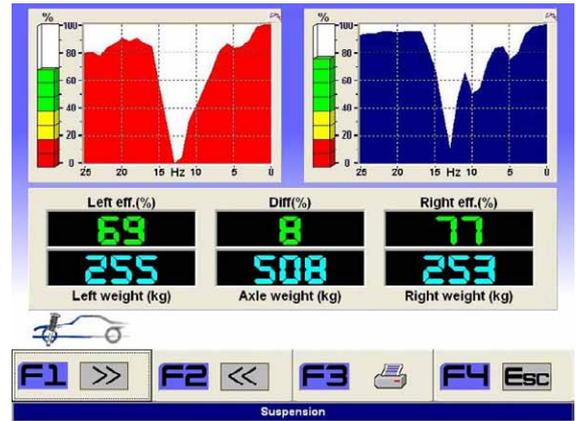
*Suspension test results of the same vehicle with the tester adjusted to show an average efficiency value.*
