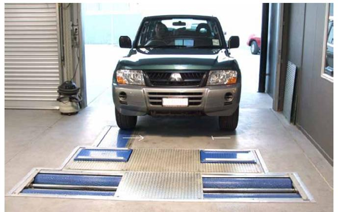
*VTEQ side slip tester in a test lane configuration.*
