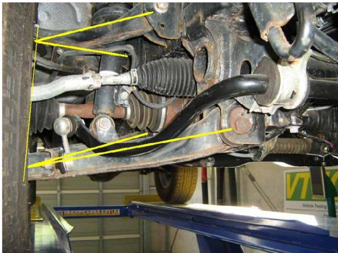
*Highlighted in yellow are the lines of the top and bottom wishbone and the king pin*
