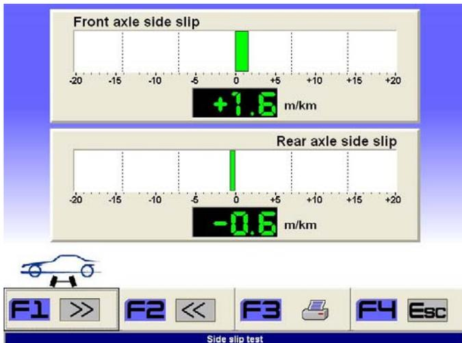
*Readings with acceptable non modified wheel alignment.*
