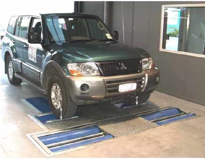
A different description for this EUSAMA (EUropean Shock Absorber Manuf. Association) type suspension tester is 'road contact tester'.
