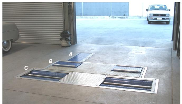
*A = Sideslip tester, B = suspension tester, C = Brake tester*
