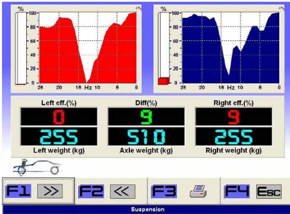
*Suspension test results of a well balanced vehicle with new 'sports' suspension, note the efficiency.*
