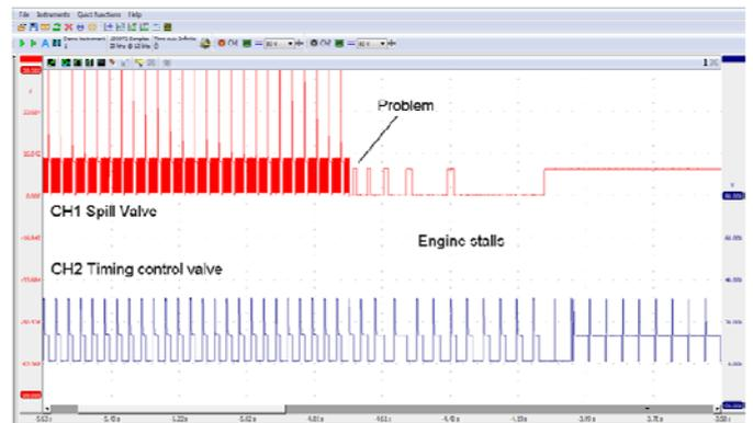
*ATS scope recording with the new multi-channel software when the problem occurred*
