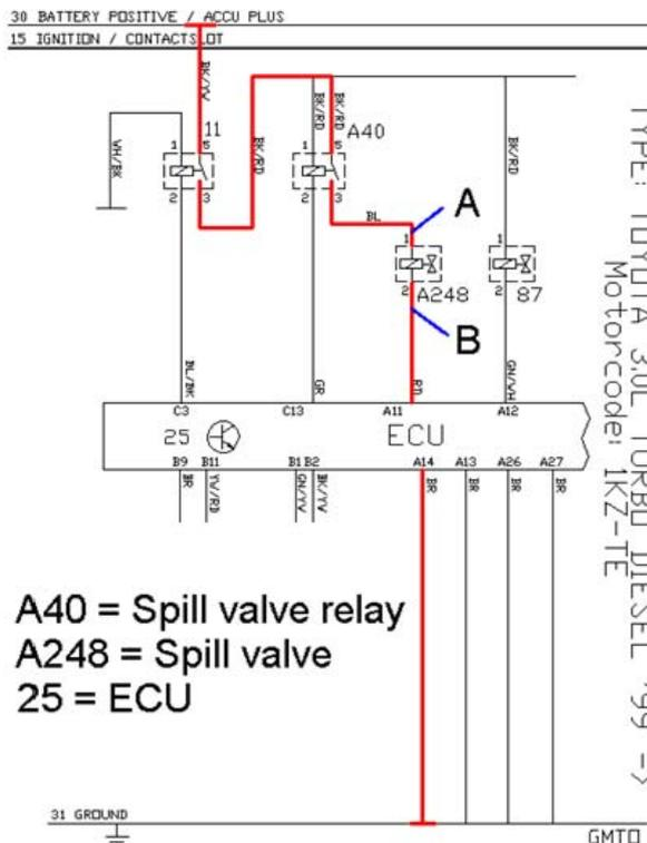
A40 = Spill valve relay
