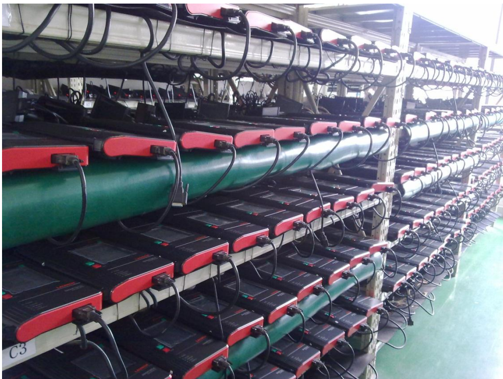
Launch Master X431 post production continuous testing rig
