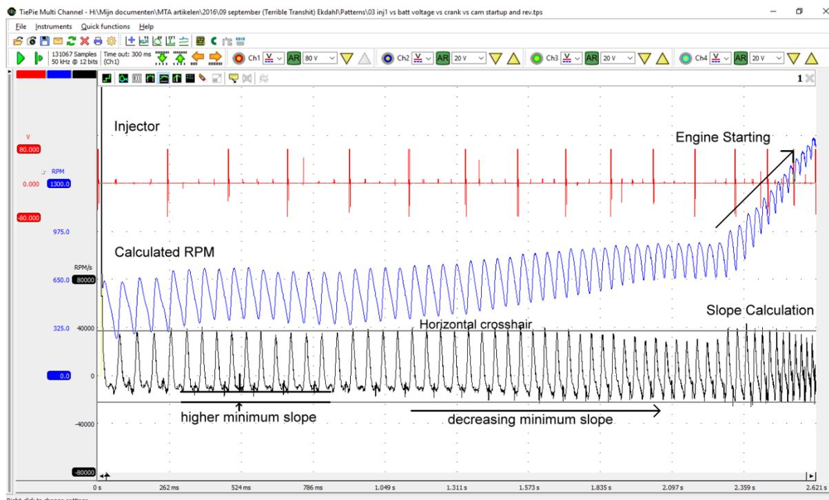
Figure 3: injection vs. calculated RPM showing the slope calculation.
