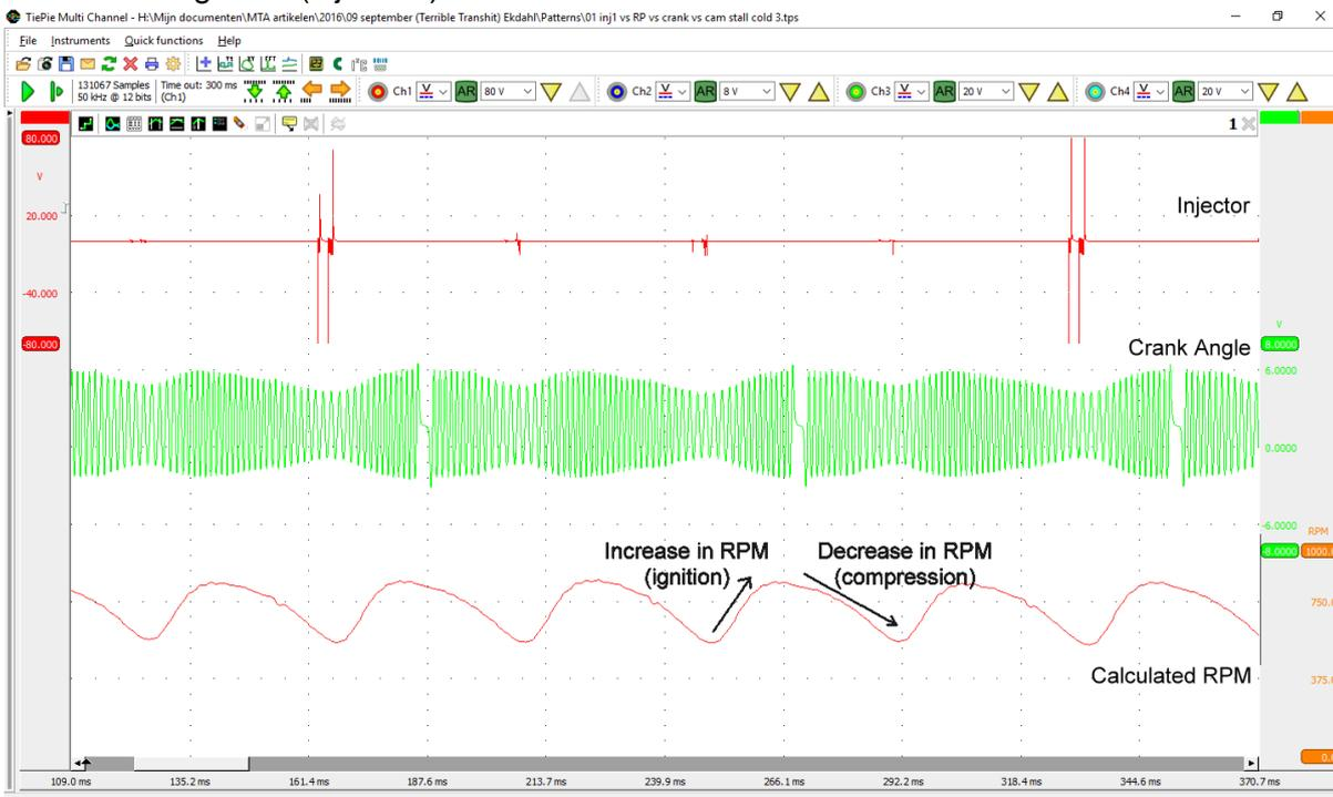
Figure 2: visual comparison of Delta-N (RPM) slopes.
