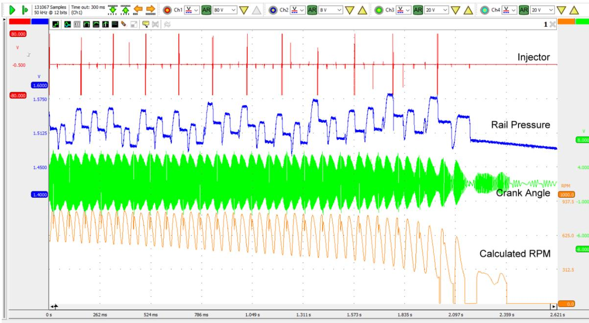
Figure 1: Injector, rail pressure, crankshaft and calculated RPM during the engine stalling.
