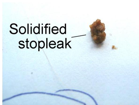
*Solidified Stopleak we found in many pipes and orifices inside the A/C service equipment.*
