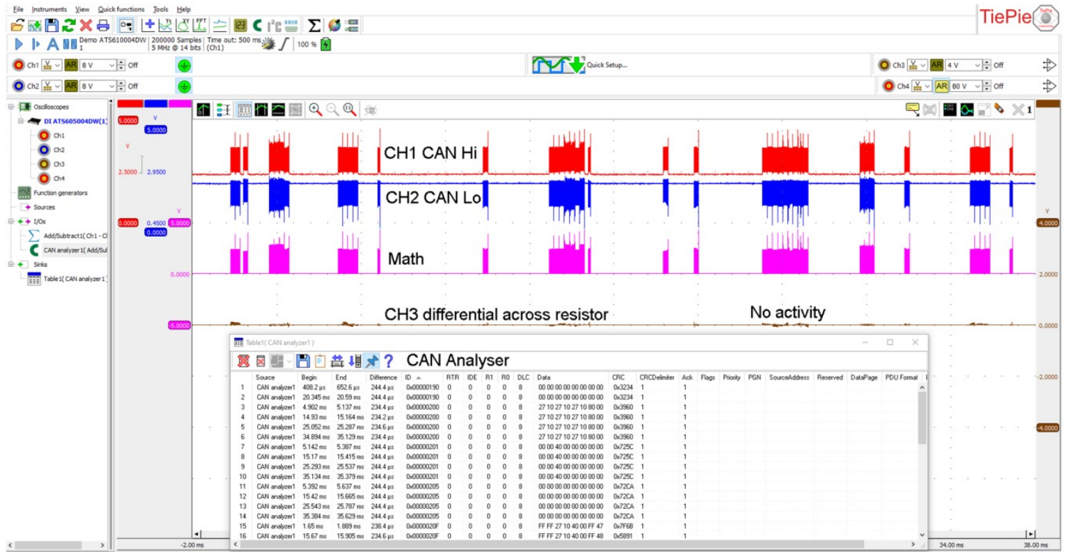
This recording clearly showed on CH3 that no data was sent from the TCM onto the CAN bus.
