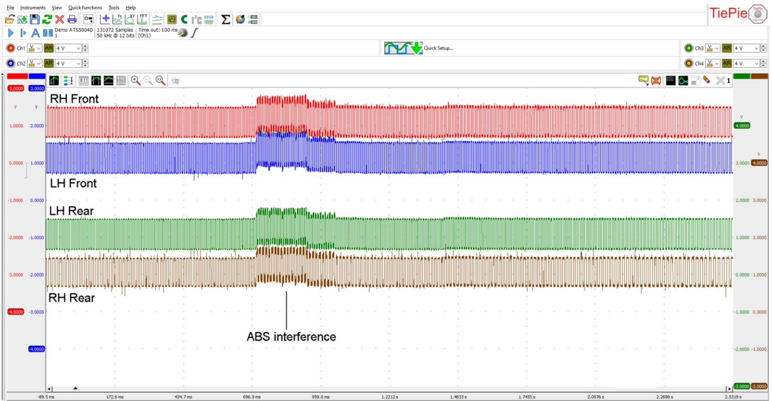
ATS scope recording made while cornering when the stability control function of the ABS changed the car's direction unintended.
