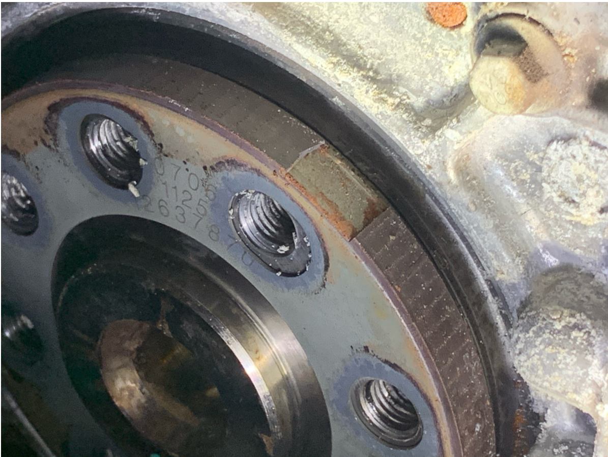
Magnetic tape tone wheel of the Colorado, spot the missing piece.
