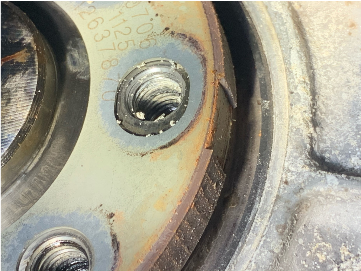
Close up detail of the damaged tone wheel
